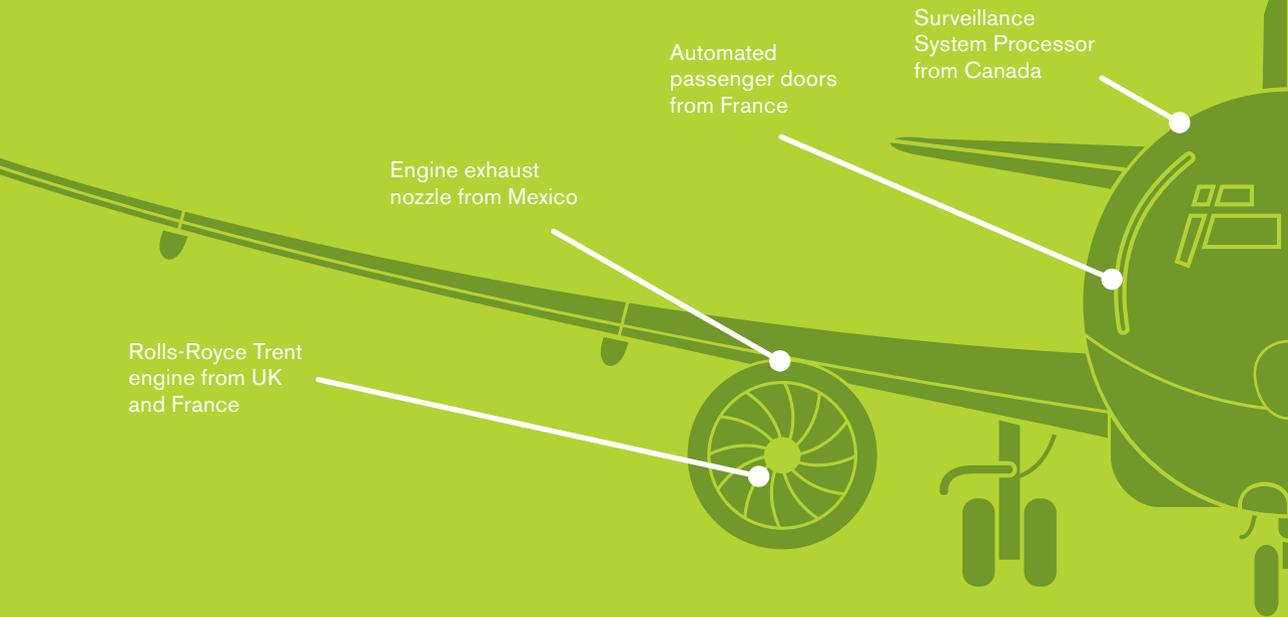
There’s the Integrated Surveillance System Processor and an Integrated Navigation Radio, from Canada.
